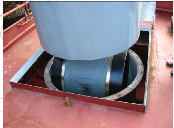
The 100 kW prototype have a flange mounted trunk to enable installation with the ship afloat.
